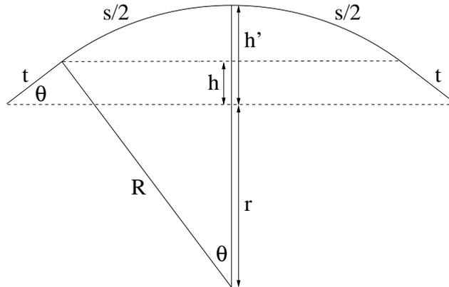
**Figure 4.** Geometry of the actuator with tabs.
