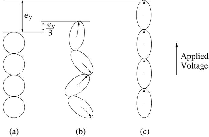
**Figure 3.** Material behavior of the PZT wafer as it is cooled through the Curie temperature (after Jiles [9]). (a) Material in the paraelectric regime above the Curie temperature; (b) Random domain structure below the Curie temperature; (c) Saturation polarization due to an applied voltage.
